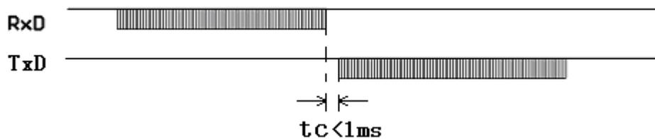
**b. The delay time of transceivers between the first bit sent by TxD to the first bit received by RxD.**
